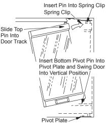
Figure 35 - Installing Optional Glass Door
